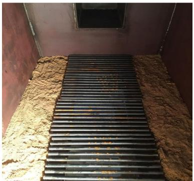
the furnace is set on the pad. There will be four plates and the bolts to mount them sent with the furnace. Usually, the delivery driver will have these plates along with any other loose items that come with the furnace. Prior to firing your furnace put sand in the open areas on both sides of the furnace grates and install the fork port covers.
